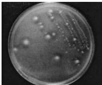
Fig. 1. Colonies of Saccharothrix waywayandensis JCM 9114 and clear zones formed on an agar plate with emulsified PLA.
